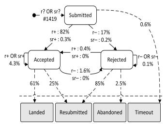
Figure 3. Patch lifecycle for core contributors for post-rapid release time.
