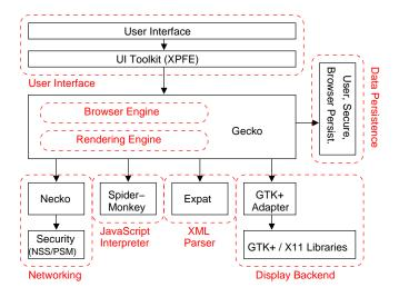
Figure 4. Architecture of Mozilla
