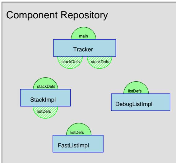
Figure 1: A simple repository. The blue boxes represent program units. The green “tab” on the top indicates the interface the unit implements. The green “slots” (striped tab) indicated the required imports.
