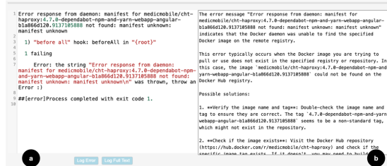
Fig. 2. Partial view of the LogExp tool's interface. The log is displayed on the left, allowing participants to choose between viewing a summary or the full log. On the right, the corresponding textual explanation generated by the LLM is presented. Below these sections, participants encountered statements and questions specific to each case.
