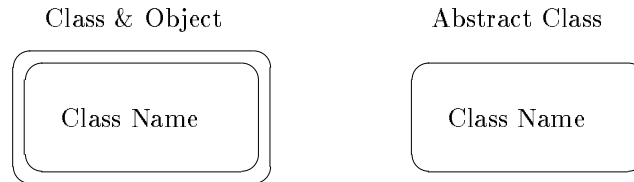
Figure A.2: Class and Object Simplified Notation
